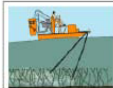
Figure 1. Bottom acre-foot treatment, with trailing weighted hoses. This system delivers the herbicide directly into the weedbed for maximum efficiency and lower cost.
