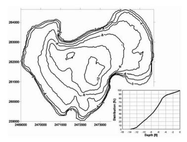
Figure 2. Bathymetric contour map from survey 2 with depth distribution graphic insert.
