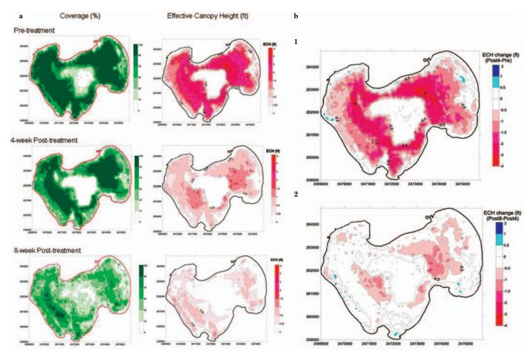
Figure 3a. Coverage (%) and effective canopy height (ft) for all 3 surveys (could be gray or color). Figure 3b. Change detection of ECH generated by subtracting the pre-treatment gird from the 4-week post-treatment gird (1), and the 4-week post treatment gird from the 8-week post treatment gird (2).
