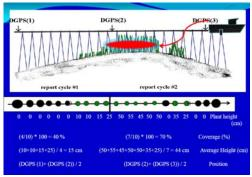
stamped, geo-referenced and digitally stored. This system allows for the data to be collected during treatment, so real time plant data is available to support post treatment efficacy evaluations.
