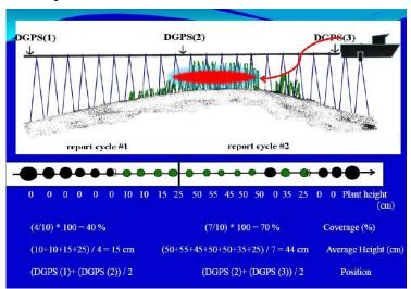
System (Littoral Zone Treatment Technology) with ERDC-EL Hydroacoustic Submersed Plant Mapping capabilities (SAVEWS<sup>TM</sup> and related developments). It is envisioned that these two technologies will be used together to achieve precision application of herbicides to submerged, nuisance aquatic vegetation.
